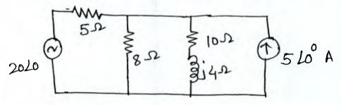
Q2a Using graph theory determine loop currents in the given network
